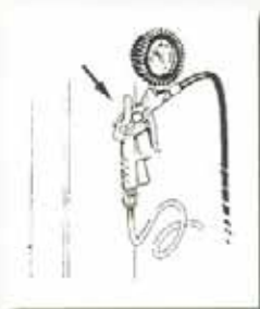
Inflation gun with manometer (cod. 100183)
